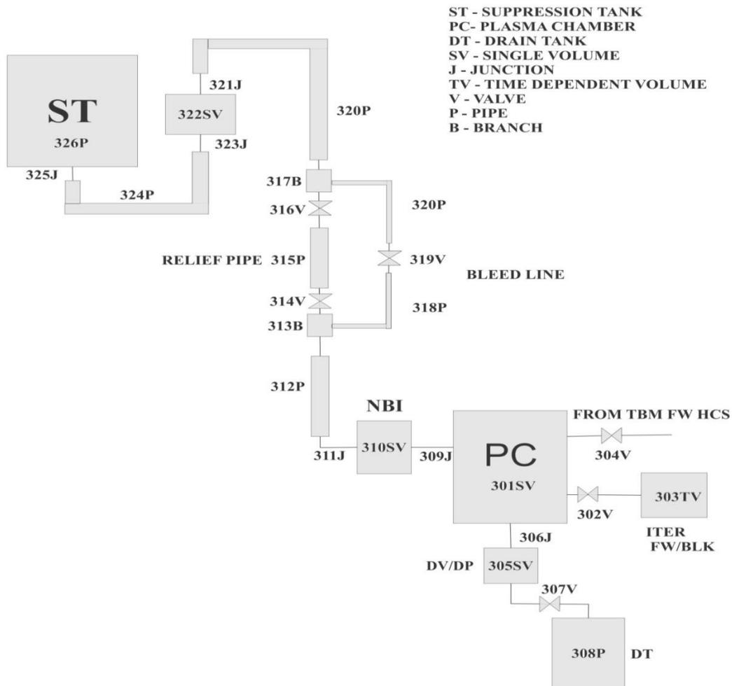
Figure 3 RELAP5 Nodalization diagram of VVPSS System.
