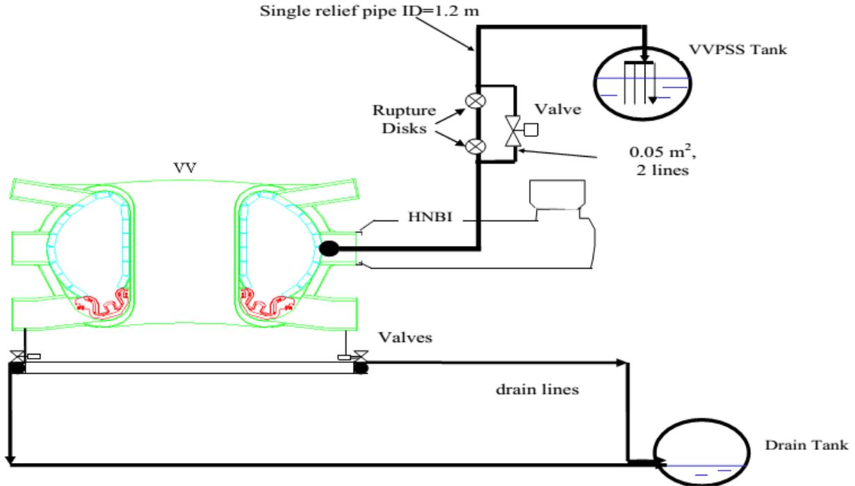
Figure 2 ITER VV and VVPSS assembly.
