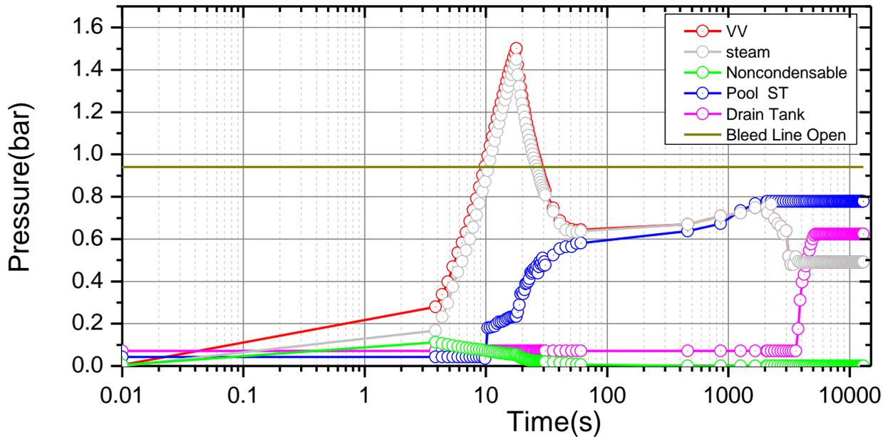
Figure 4 VV and VVPSS Pressure Profile In-Vessel TBM Coolant Leak case.
