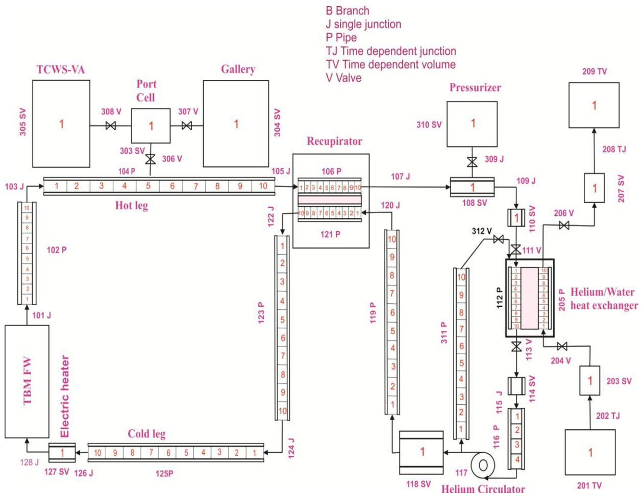
**Fig.1.** Thermal hydraulic nodalization of TBM FWHCS
