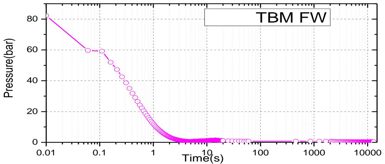
Figure 5 TBM-FW Pressure Profile In-Vessel TBM Coolant Leak case
